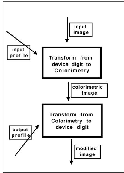
Figure 1b: Logical ICC image processing block diagram.
