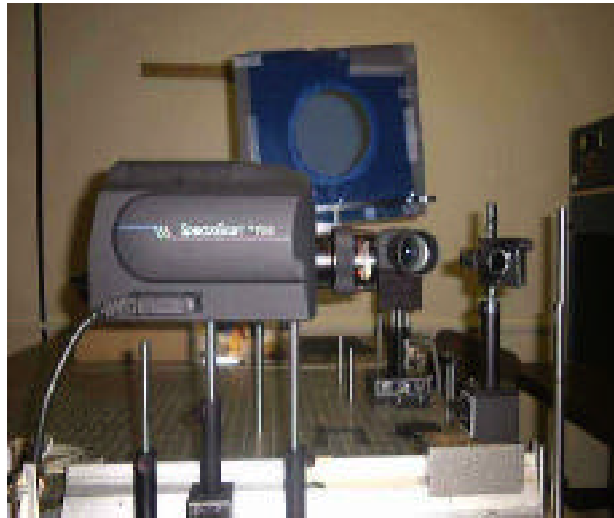
Fig. 7 Picture main parts of imaging system
