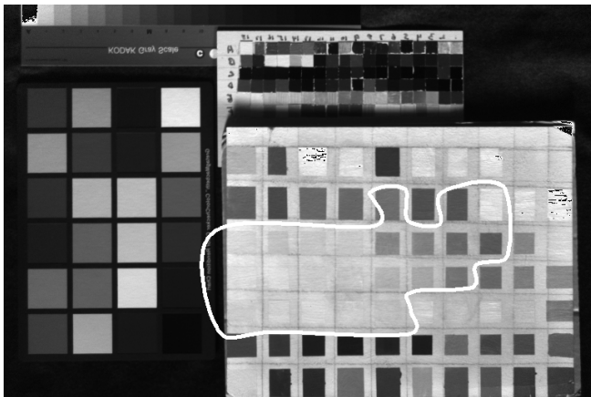
Figure 11. Narrow-band patches used for creating system model with best average results. 23 circled patches comprise the set.
