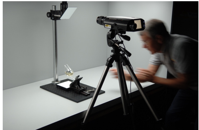
FIGURE 1. The experimental setup for in situ (ISO tasting glass) wine transmittance measurements.
