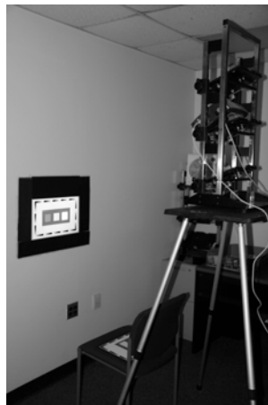
Figure 2. The experimental setup of the SL1 experiment in a dark room. The area outside the configuration was illuminated by the camera flash, but was dark during the experiments.
