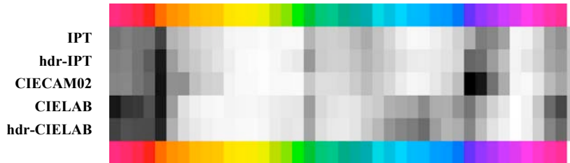
Figure 11. Visualization of PCA analysis on the dimensionality of constant hue lines. Dark entries indicate that a significant amount of variation requires two dimensions to describe (an indication of hue nonlinearity). (The first and last rows are the representative colors of the hue angles form 0° to 351° at an interval of 9°.)
