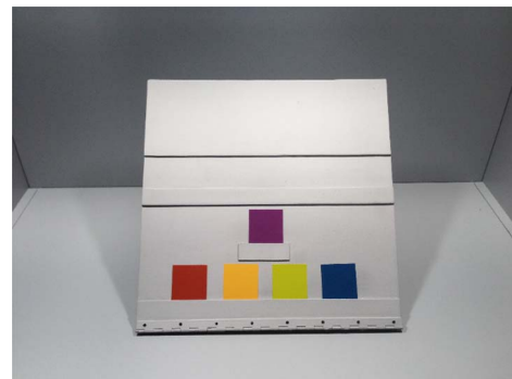
Fig. 4. Visual assessment involving 45/0 illumination viewing geometry, and a custom made sample stand painted in neutral gray that housed the standard and test samples.
