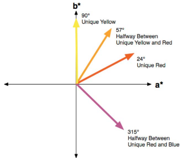
FIG. 2. Anchor hues chosen in the CIELAB color space for the chromatic noise adjustment experiment.
