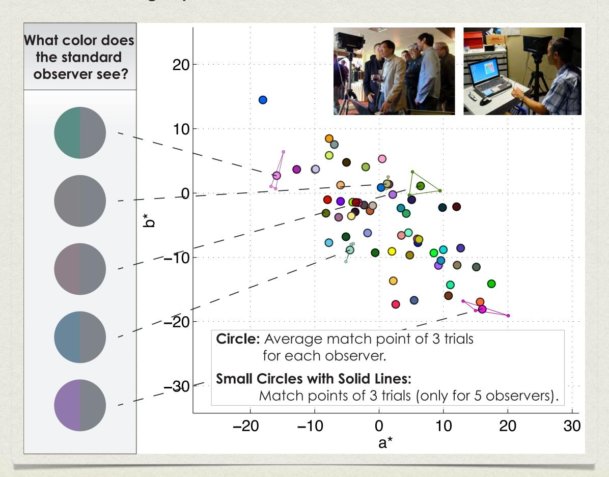
The individual differences in color matching functions (CMFs) can be a serious issue in industries especially when spectrally narrow stimuli such as LEDs and lasers are viewed. To capture individual differences in CMFs efficiently, we designed a color matching experiment to magnify interobserver variability.
