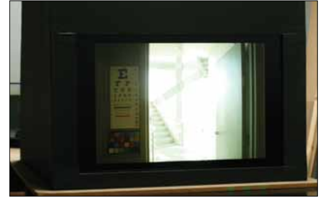
Prototype dual modulator HDR display with high dynamic range content.
