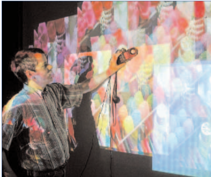
Dave Wyble posing with his video projector color measurement setup. While it is a pretty picture, unfortunately he couldn't really measure them all at once and the actual test targets were less interesting visually.
